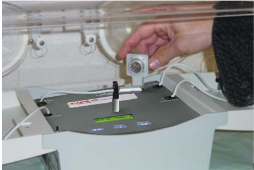
*Figure 3-5. Placement of Air Flow Sensor*
