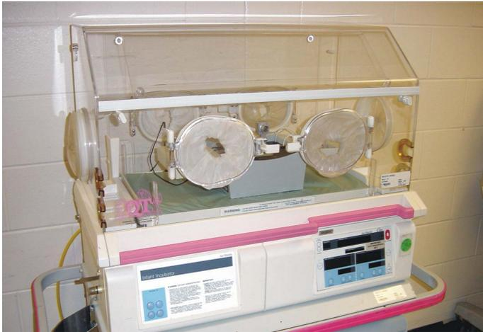
*Figure 1-1. Closed incubator with forced convection*
