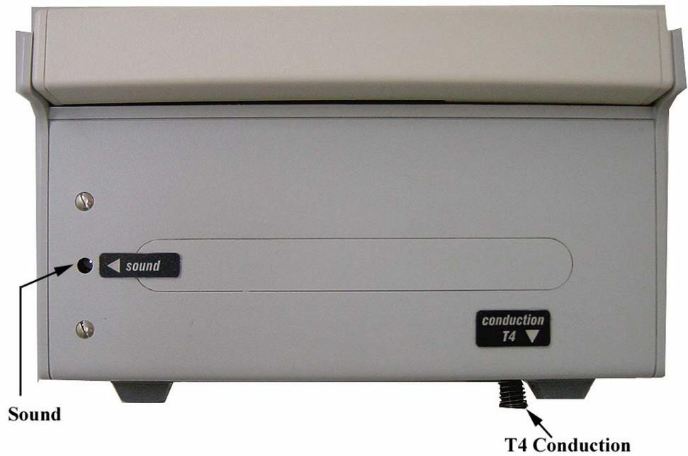
*Figure 3-6. Placement of temperature sensor T4*
